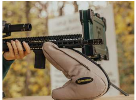
VELOCIRADAR SLIGHTLY BEHIND MUZZLE.
